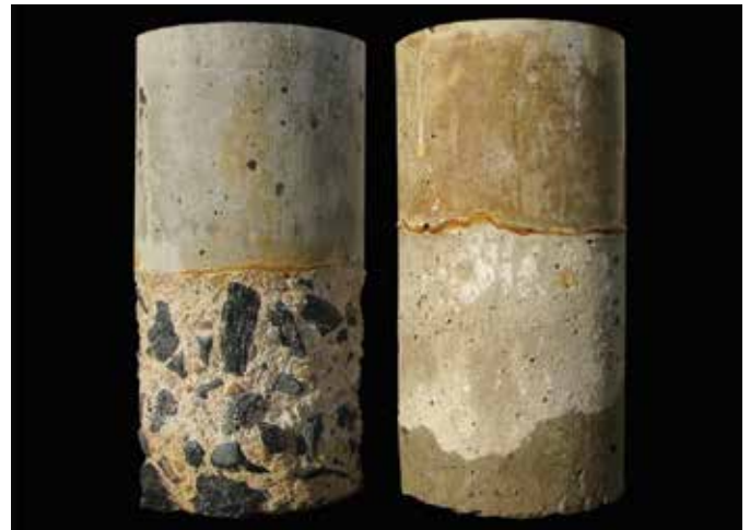
Fig. 2: These 4 x 8 in. (100 x 200 mm) concrete cylinders were partially submerged in a 15% sulfuric acid solution for 28 days per ASTM C267. The cylinder produced using OPC (left) exhibited significant corrosion, exposing the coarse aggregate. The cylinder produced using activated fly ash cement concrete (right) exhibited only minor damage
